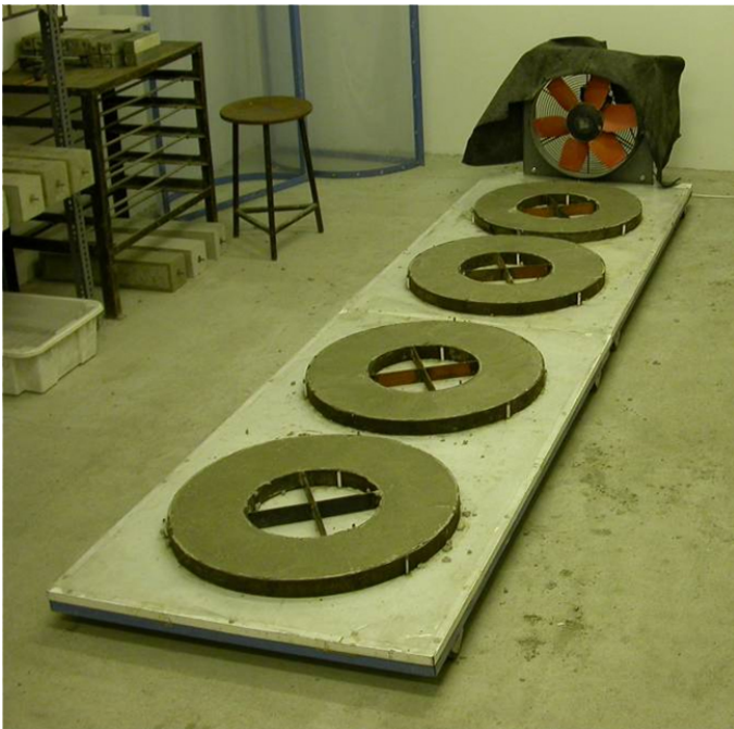
Fig. 5. Empty wind tunnel with ring specimens according to the Austrian fibre-concrete technical specification [16, 17]
