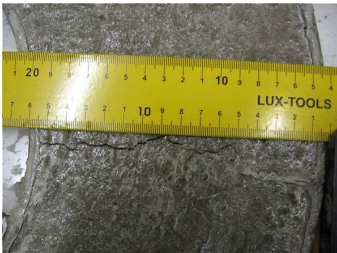
Fig. 8. Measuring crack length on a ring specimen after testing [19,27]
