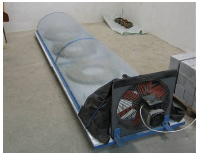
Fig. 6. Wind tunnel with ring specimens according to the Austrian fibre-concrete technical specification [16, 17, 19, 27]
