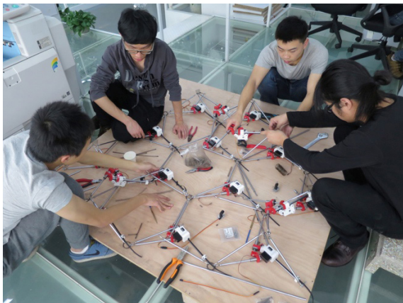
Fig. 27 Assembly of units on the stable base
