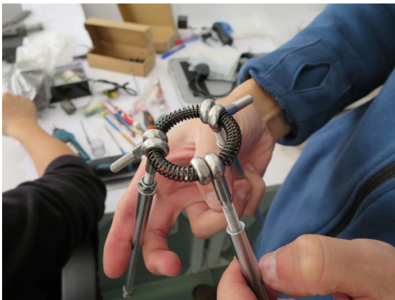
Fig. 16 The universal rotating joints
