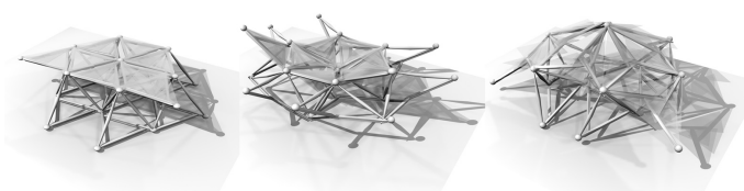
Fig. 17 The digital transformation of concave and convex caused by a sliding motion at the top and bottom layer
