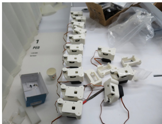
Fig. 23 3D print sliding joints
