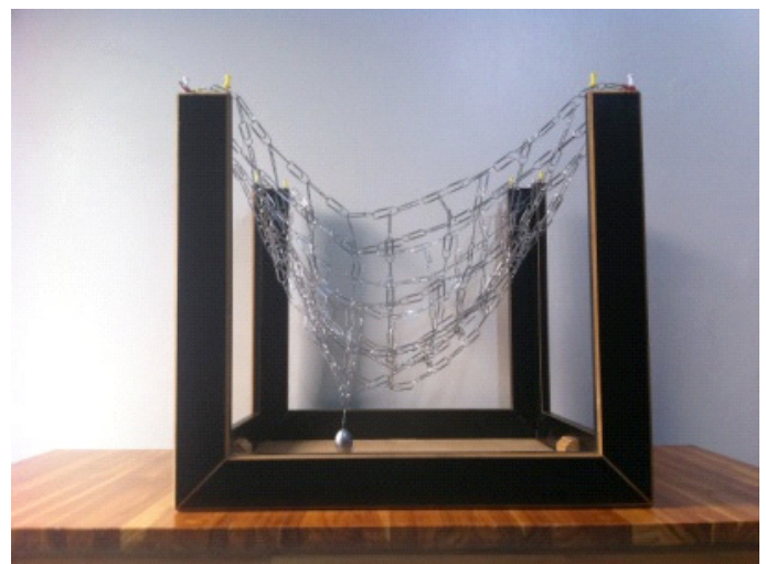
Fig. 5 Experiment performed with different meshes and using a weight to test their manipulation (Makert, 2015)
