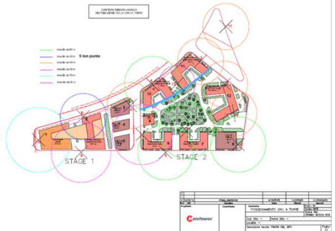
Fig. 7 Tower cranes layout proposed by the crane renting company and General Contractor
