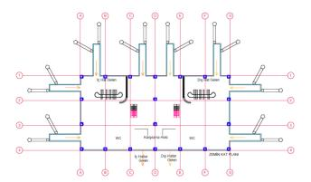
Fig. 4 Designed Airport Terminal Building Ground Floor Plans
