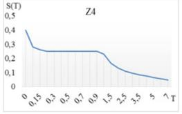
Fig. 6 Spectrum Curve for the Z4 ground class.
