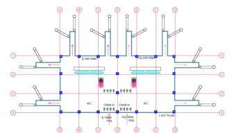
Fig. 5 Designed Airport Terminal Building First Floor Plans
