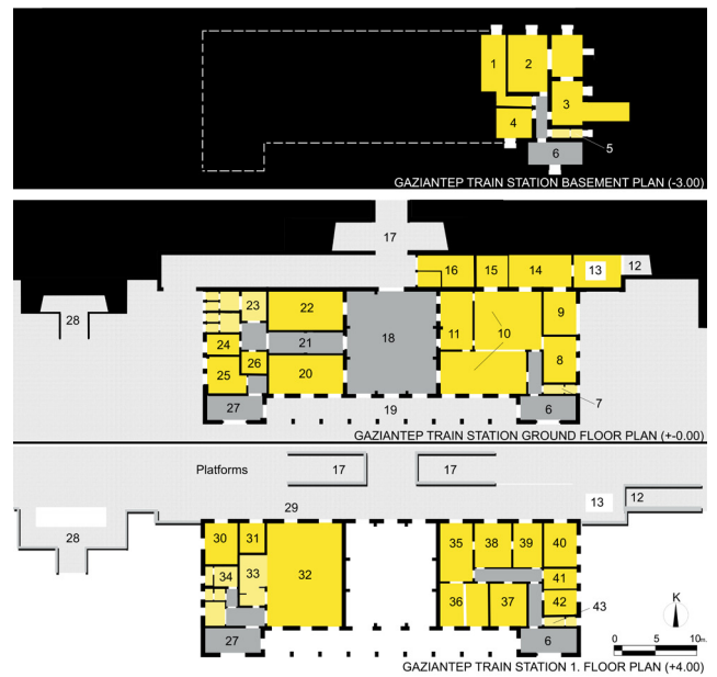
Fig. 16 Gaziantep Train Station Floor Plans: 1. Technical Room, 2. Tank, 3. Boiler Room, 4. Technical Room, 5. WC, 6. Staircase, 7. WC, 8. Room, 9. Room, 10. Luggage Room, 11. Ticket Counter, 12. Staircase to platforms, 13. Elevator, 14–16. Room, 17. Staircase to platforms, 18. Passenger Lounge, 19. Main Entrance, 20. Room, 21. Corridor, 22. Room, 23. WC, 24. Room, 25. Kitchen, 26. Depot, 27. Staircase, 28. Staircase to platforms, 29. Staircase to platforms, 30–31. Room, 32. Dining Hall, 33. Kitchen, 34. WC, 35–42. Room, 43. WC.
