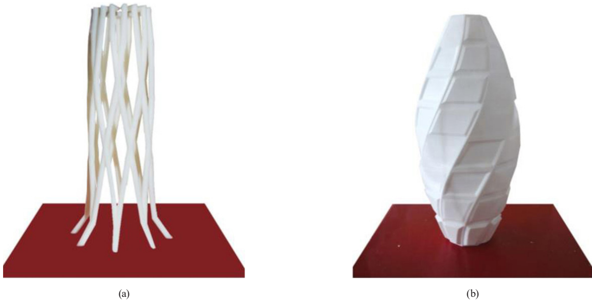
Fig. 7 Collection of (a) SLA and (b) FDM 3D printed columns
