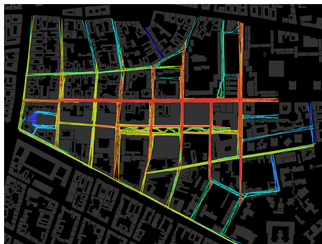
Fig. 7 Space syntax model of axial analysis of the space after development of the area
