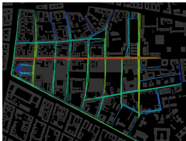
Fig. 6 Space syntax model of axial analysis of the space before the development of the promenade
