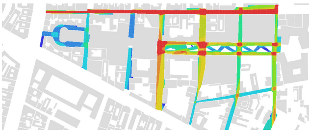
Fig. 8 Isovist area of visible space: the area of visible space from each cell is proportional to the number of cells directly visible from each cell. (Red: More isovist area, Blue: Less isovist area)
