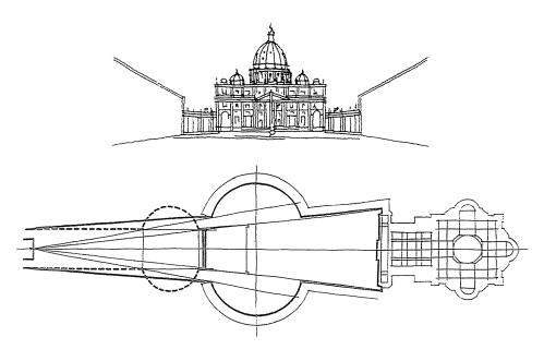
Figs 12—13. Disclosure of the square system from the entrance to the third square part. (The perceptible square form in dash line in the ground plan)
