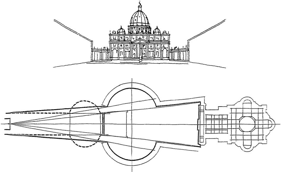
Figs 12—13. Disclosure of the square system from the entrance to the third square part. (The perceptible square form in dash line in the ground plan)
