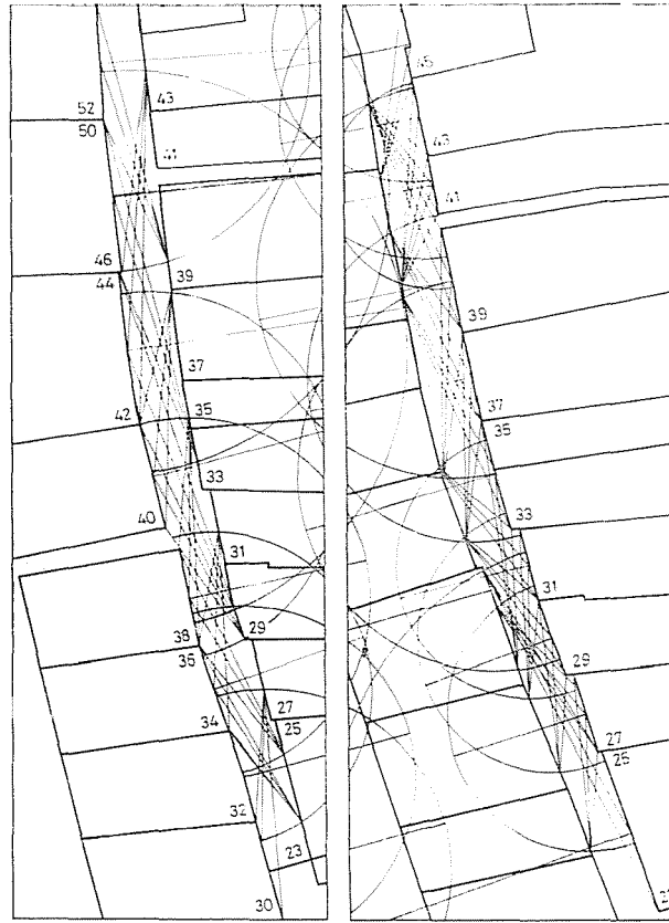
Fig. 5. Construction of optimum looking points to houses of a part of Uri street. Intersections of arc two and half times the façade width with the street line are the nearest points the façade can be overlooked from. To consider the street as narrow or wide compared to the façade dimensions is decided by the looking angle and so is the accent to be borne by walls or courses
