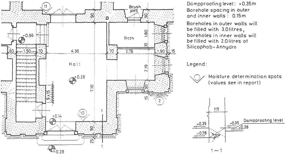
Fig. 4. Detail of a wall dampproofing plan
