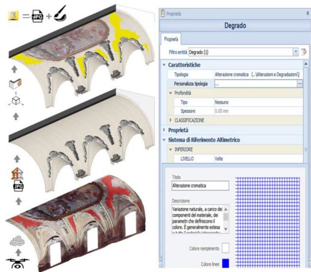
Fig. 8 Church of San Pietro in Vinculis, Naples: mapping of the decay on the vaults using Edificius software (Lanzara et al., 2021). The properties associated in this table with the parametric object describe type of decay, thickness, altimetry reference system, description, pattern
