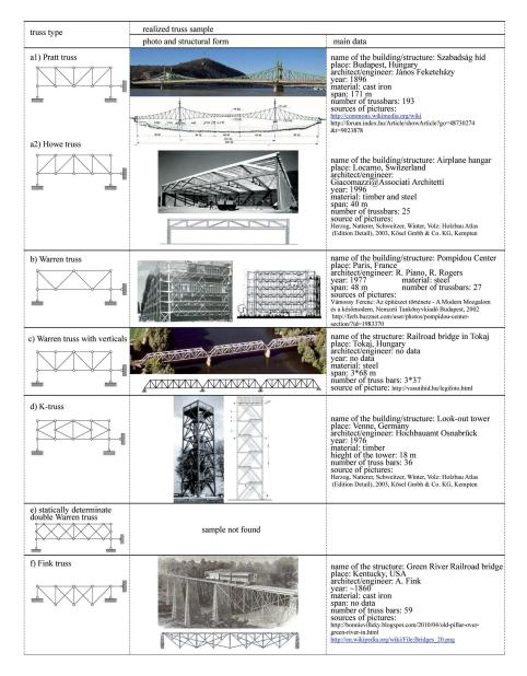
Fig. 6. Topology types belonging to the class of simple trusses.
