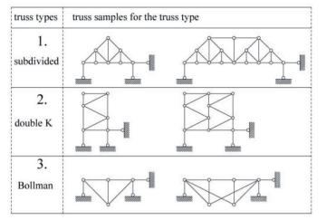
**Fig. 5.** Topology types which also have simple (see the first samples) and compound (see the second samples) truss representatives.
