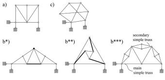
**Fig. 3.** Examples for the truss classes after Hibbeler: simple truss (a), compound truss (b figures), complex truss (c).
