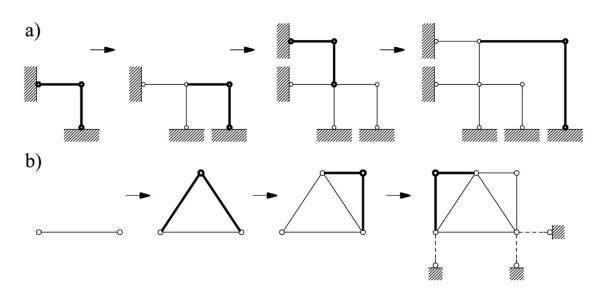
Fig. 2. Two ways of generating simple trusses.
