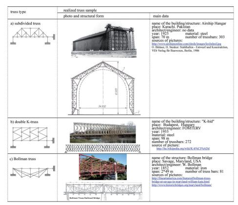
Fig. 7. Topology types, in which almost all elements of the type are compound trusses.
