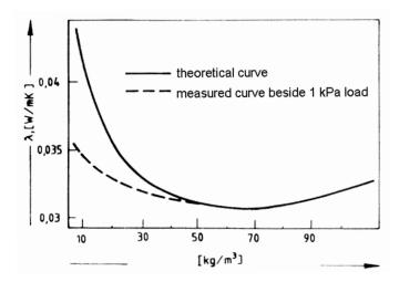
Fig. 8. The thermal conductivity factor of glass wool as a function of density [9, p. 104].
