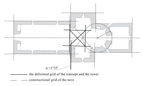
Fig. 4 The constructional grids of the church
