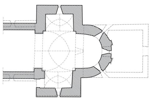
Fig. 11 The hypothetical reconstruction of the church's original plan compared to its present state
