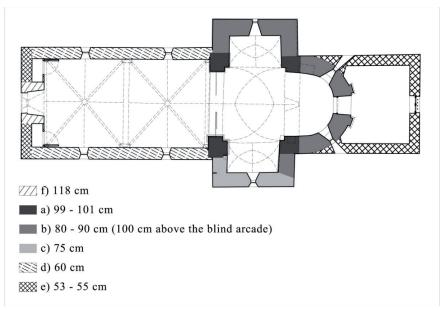
Fig. 5 The different wall thicknesses
