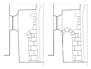
Fig. 7 The remnant of the southern doorway in the southern transept (as seen from the interior) and the theoretical reconstruction of the original form
