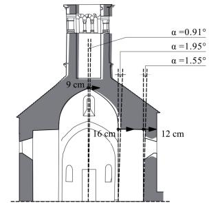
Fig. 6 Comparison of the current cross section with its hypothetical original undeformed state
