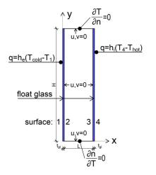
Fig. 22 Schematic representation of the glazing system geometry and boundary conditions
