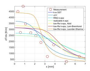
Fig. 13 Temperature gradient normal to the cold wall at y/H=0.5 [-]
