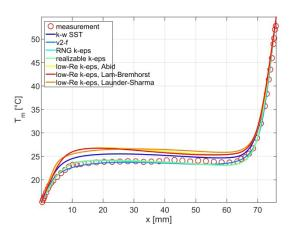
Fig. 4 Horizontal T<sub>m</sub> profile at y/H=0.05 [-]
