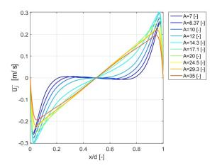
Fig. 17 Horizontal profile of mean vertical velocity at y/H=0.5
