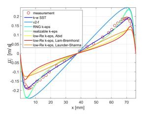
Fig. 9 Horizontal profile of mean vertical velocity at y/H=0.50 [-]
