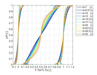
Fig. 23 Horizontal temperature profile in the cavity
