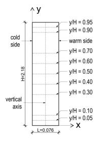
Fig. 2 A schematic representation of the 'natural convection in a rectangular differentially heated cavity' problem
