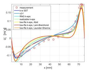
Fig. 8 Horizontal profile of mean vertical velocity at y/H=0.05 [-]
