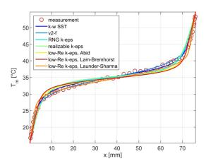
Fig. 5 Horizontal T<sub>m</sub> profile at y/H=0.50 [-]
