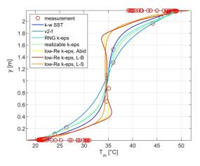
Fig. 7 Vertical T<sub>m</sub> profile
