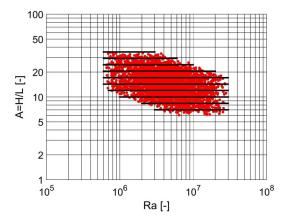
Fig. 14 The typical flow regime in cavities of box type windows (indicated with pairs of Ra and A numbers) and the range of the current study
