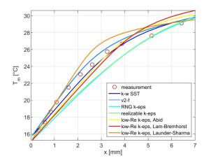
Fig. 12 Temperature field normal to the cold wall at y/H=0.5 [-]
