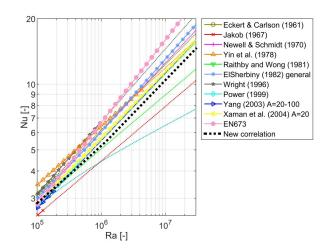
**Fig. 21** Comparison of the new correlation for the Nusselt number with the ones found in the literature, for A=20 [-] (each correlation is plotted as continuous for its published range of validity and with a dotted line outside the range)
