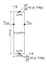
Fig. 3 The cavity geometry and boundary conditions
