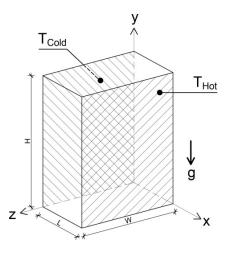
Fig. 1 A schematic representation of the 'natural convection in a rectangular differentially heated cavity' problem
