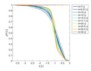
Fig. 18 Relative distribution of heat flux density along the height of the cold cavity wall
