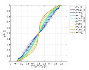
Fig. 16 Vertical temperature profile in the cavity axis for high Ra (solid) and low Ra (dashed) simulations
