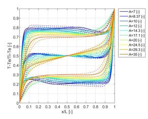
Fig. 15 Horizontal temperature profiles at y/H=0.1,0.5 and 0.9, for high Ra (solid) and low Ra (dashed) simulations
