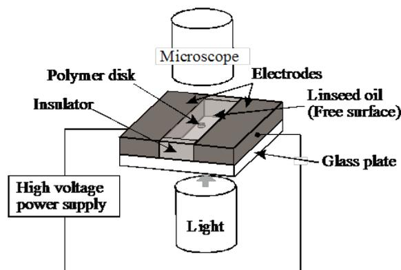
Fig. 1 Experimental set up to determine the dependence of rotational speed on the DC field intensity.
