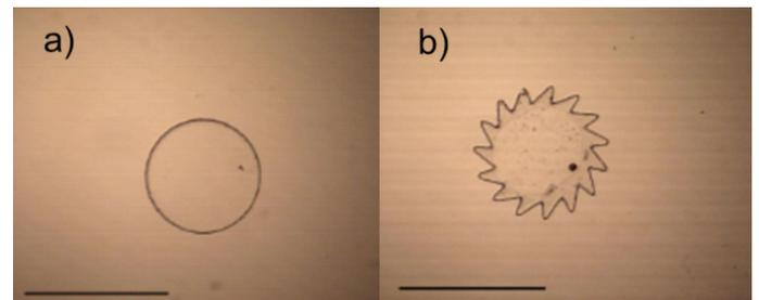
Fig. 4 Polymer rotor prepared from epoxy based polymer. (a) disk, (b) gearwheel. The bar indicates 500 microns. The dot close to the edge of the micro tools was used to determine the speed of rotation.
