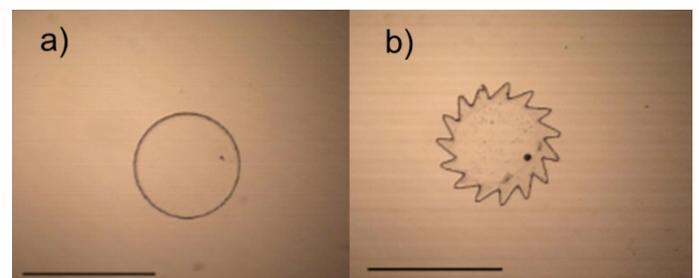
Fig. 4 Polymer rotor prepared from epoxy based polymer. (a) disk, (b) gearwheel. The bar indicates 500 microns. The dot close to the edge of the micro tools was used to determine the speed of rotation.
