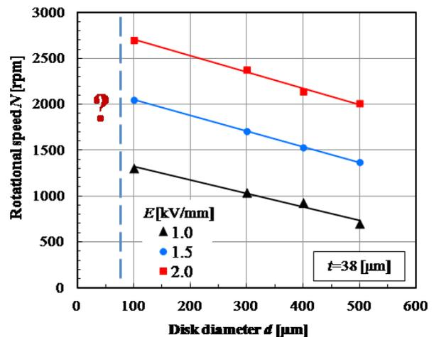
Fig. 3 Dependences of rotational speed  $N$  on the diameter  $d$  polymer disks
