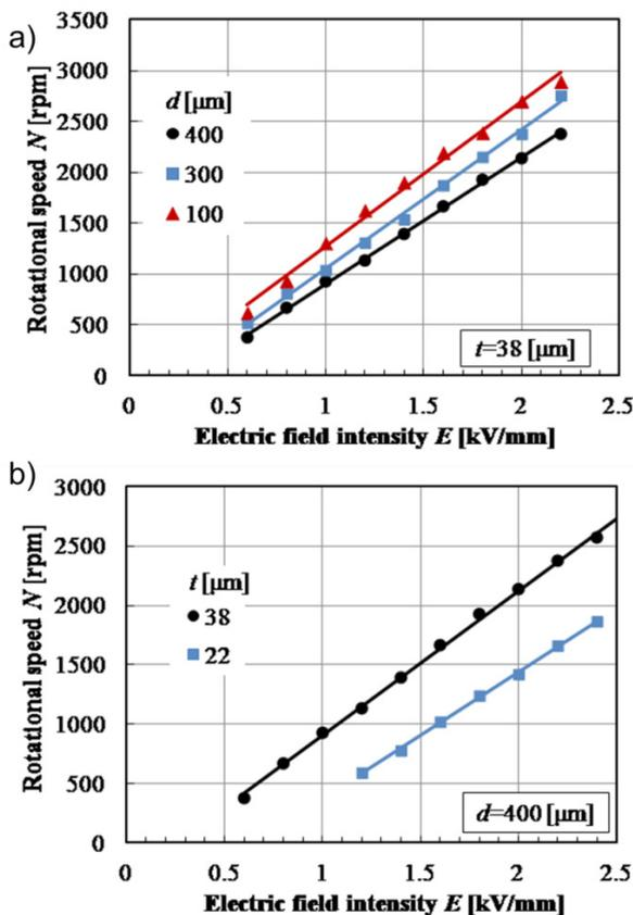
Fig. 2 Dependences of rotational speed  $N$  on the diameter  $d$  (a) and thickness (b) of polymer disks.
