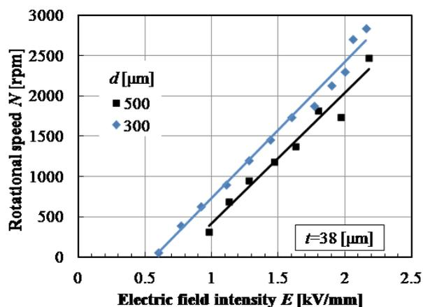
Fig. 5 Dependence of rotational speed  $N$  of polymer gear wheels as a function of electric field intensity  $E$  on the diameter  $d$ . The thickness of the gears is  $t=38 \mu\text{m}$ .
