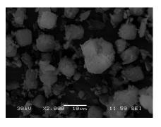
Fig. 1 SEM image of the catalyst
