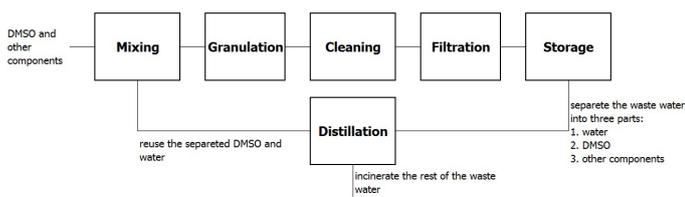
Fig. 3 The planned manufacturing process (closed technology)
