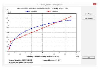
Fig. 6 Graphical result of fit Solubility Limited Leaching Model
