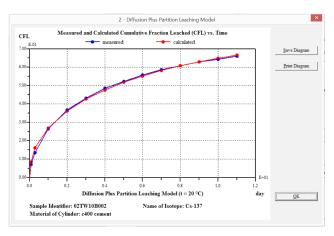
Fig. 5 Graphical result of fit Diffusion Plus Partition Leaching Model
