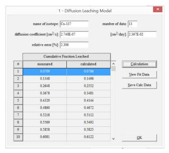
Fig. 3 Calculation results choosing the "Diffusion Leaching Model"
