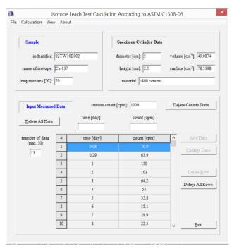
Fig. 1 Input leach test data of cemented evaporator bottom residue of tank 02TW10B002
