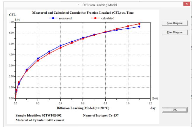
Fig. 4 Graphical result of fit Diffusion Leaching Model
