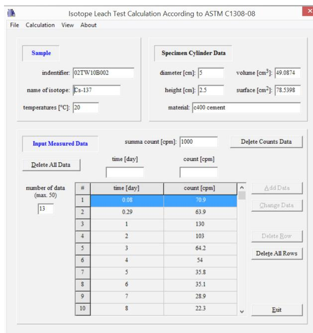
Fig. 1 Input leach test data of cemented evaporator bottom residue of tank 02TW10B002
