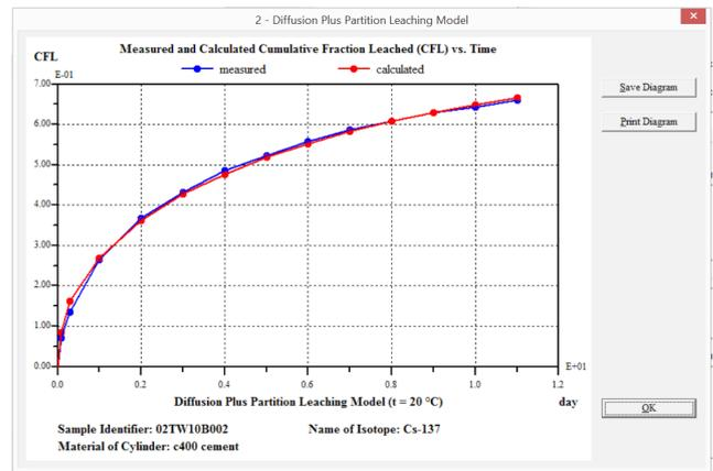
Fig. 5 Graphical result of fit Diffusion Plus Partition Leaching Model
