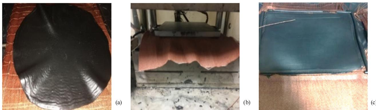
**Fig. 3** Production of Cord Fabric/ NR-NGP composite materials: a) Preformed thin NR/NGP sheet before curing b) Cord fabric coating process under hot pressing in a mold c) Vulcanized Cord Fabric/NR-NGP composite plate.
