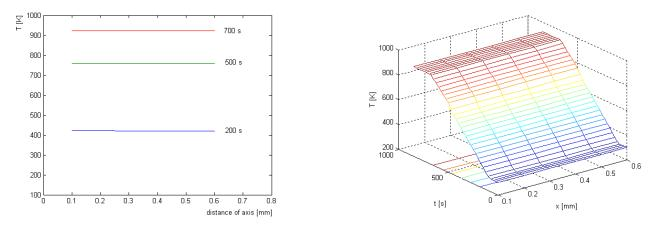
Fig. A.6 Temperature profile as a function of reaction time and position Case III: heating rate 55 K/min
