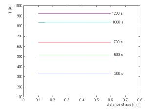
Fig. 5 Temperature profile as a function of position Case II: heating rate 32 K/min
