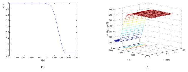
Fig. A.1 Mass loss of wood sample: (a) as a function of reaction time, (b) as a function of reaction time and position Case I: heating rate 21 K/min
