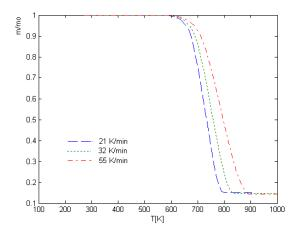
Fig. 3 Mass loss of wood sample as a function of temperature and heating rate
