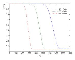
Fig. 2 Mass loss of wood sample as a function of reaction time and heating rate
