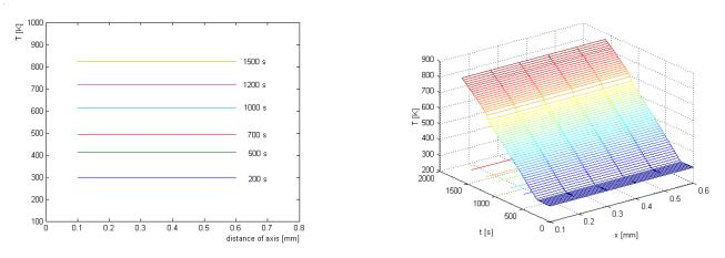
Fig. A.4 Temperature profile as a function of reaction time and position Case I: heating rate 21 K/min
