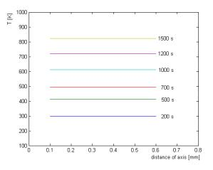
Fig. 4 Temperature profile as a function of position Case I: heating rate 21 K/min
