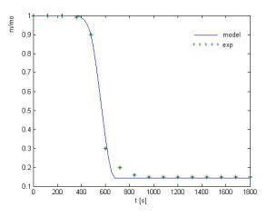
Fig. 10 Mass loss of wood sample as a function of reaction time and heating rate: 55 K/min for model and experiment
