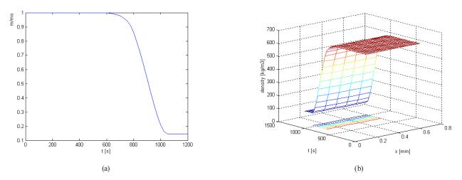
Fig. A.2 Mass loss of wood sample: (a) as a function of reaction time, (b) as a function of reaction time and position Case II: heating rate 32 K/min
