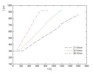
Fig. 7 Temperature profile as a function of reaction time at the center of the particleCase I: heating rate 21 K/min, Case II: heating rate 32 K/min, Case III: heating rate 55 K/min
