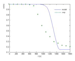
Fig. 8 Mass loss of wood sample as a function of reaction time and heating rate: 21 K/min for model and experiment
