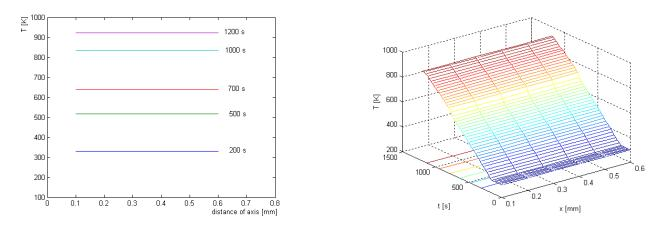
Fig. A.5 Temperature profile as a function of reaction time and position Case II: heating rate 32 K/min
