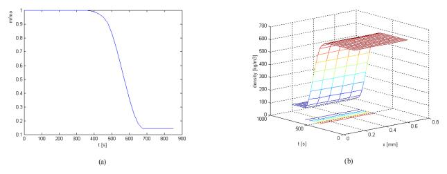
Fig. A.3 Mass loss of wood sample: (a) as a function of reaction time, (b) as a function of reaction time and position Case III: heating rate 55 K/min
