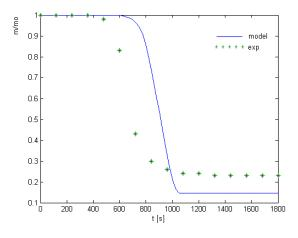
Fig. 9 Mass loss of wood sample as a function of reaction time and heating rate: 32 K/min for model and experiment
