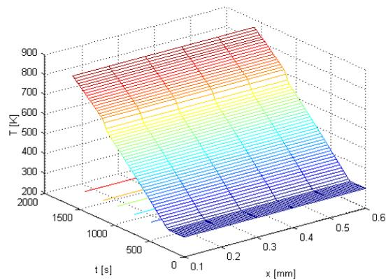
**Fig. A.4** Temperature profile as a function of reaction time and position Case I: heating rate 21 K/min
