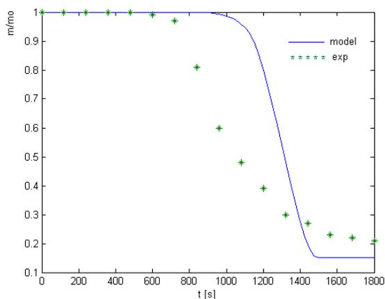
**Fig. 8** Mass loss of wood sample as a function of reaction time and heating rate: 21 K/min for model and experiment
