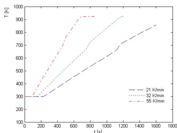
**Fig. 7** Temperature profile as a function of reaction time
