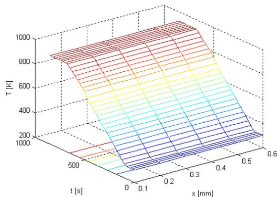
**Fig. A.6** Temperature profile as a function of reaction time and position Case III: heating rate 55 K/min
