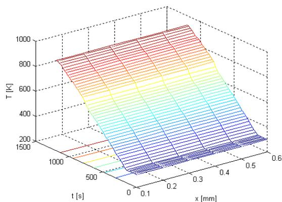
**Fig. A.5** Temperature profile as a function of reaction time and position Case II: heating rate 32 K/min
