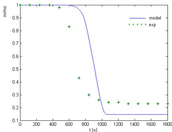
**Fig. 9** Mass loss of wood sample as a function of reaction time and heating rate: 32 K/min for model and experiment
