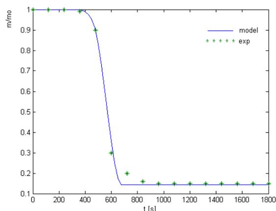
**Fig. 10** Mass loss of wood sample as a function of reaction time and heating rate: 55 K/min for model and experiment
