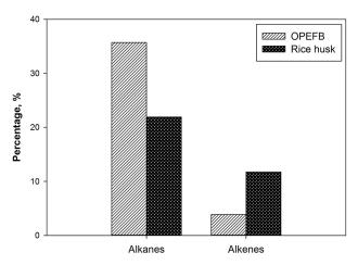
Fig. 8 Hydrocarbon distribution of bio-oil from OPEFB and rice husk
