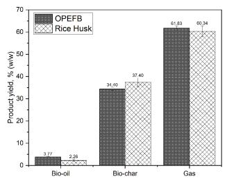
Fig. 12 Comparison of product yields between OPEFB and rice husks pyrolysis at 600 °C
