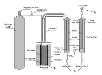
Fig. 1 Pyrolysis reactor equipment set
