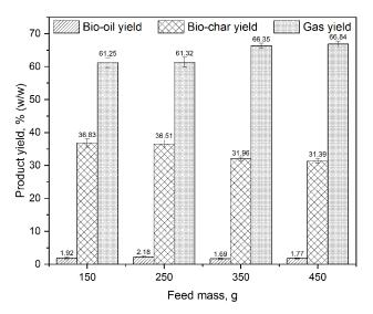
Fig. 4 Rice husk pyrolysis products yield with varied feed mass at 600 °C
