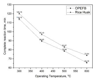
Fig. 10 Relationship between temperature with pyrolysis reaction time
