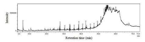
Fig. 6 Chromatogram of bio-oil from OPEFB pyrolysis
