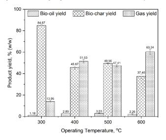
Fig. 5 Rice husk pyrolysis products yield at various operating temperature
