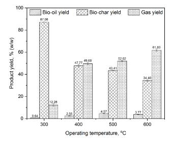
Fig. 3 OPEFB pyrolysis product yields with varied reactor temperature
