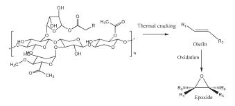
Fig. 9 Simplified mechanism of epoxide formation from biomass pyrolysis
