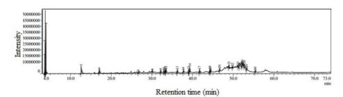
Fig. 7 Chromatogram of bio-oil from rice husk pyrolysis
