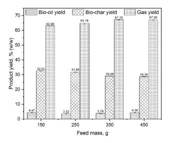
Fig. 2 OPEFB pyrolysis product yields with varied feed mass at 600°C
