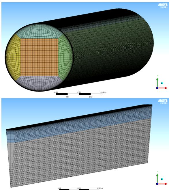
Fig. 1 The mesh of the full pipe and the  $9^\circ$  section
