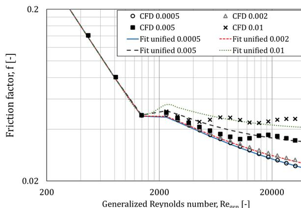
Fig. 7 Fit of the unified Colebrook-Swamee equation to the CFD results with the Bingham fluid for the rough pipes of  $\varepsilon = 0.01; 0.005; 0.002; 0.0005$
