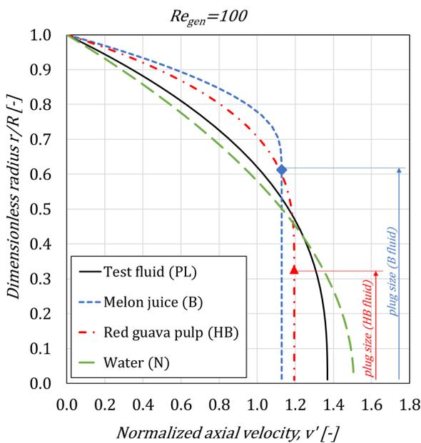
**Fig. 3** Normalized axial velocity profiles in smooth pipe for the power-law, Bingham, Herschel-Bulkley fluids and with water at  $Re_{gen} = 100$ . Analytical dimensionless radius of the flow for the B ( $r_{plug,B}/R = 0.612$ ) and HB ( $r_{plug,HB}/R = 0.326$ ) fluids
