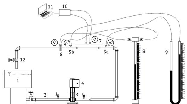
Fig. 2 The experimental setup. 1: tank, 2: pipeline system, 3: centrifugal pump, 4: electric motor, 5a, 5b: pressure taps, 6: orifice meter, 7: ultrasonic flowmeter, 8-9: U-tube manometers, 10: data acquisition device, 11: PC, 12: gate valve
