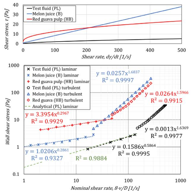
**Fig. 4** Rheograms (top) and nominal shear rate-shear stress diagrams (bottom) in smooth pipe for the three investigated fluids in laminar and turbulent regimes; the analytical curve of Eq. (12) with the power-law fluid in laminar zone (green dotted)
