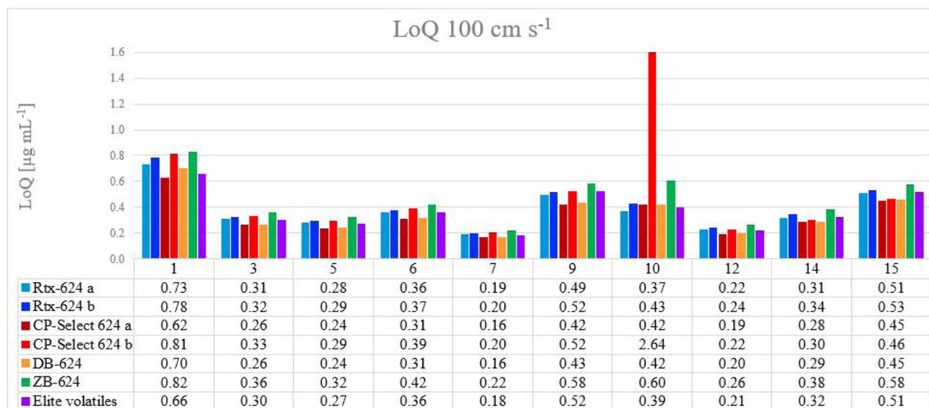
Fig. 5 Limit of quantitations of the test compounds for all investigated columns
