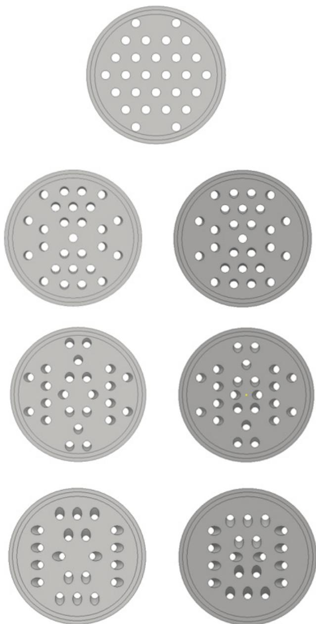
**Fig. 2** Figures of the investigated trays in top and bottom view. The figures from up to down: straight perforated, 75° inclined perforated, 60° inclined perforated, 45° inclined perforated
