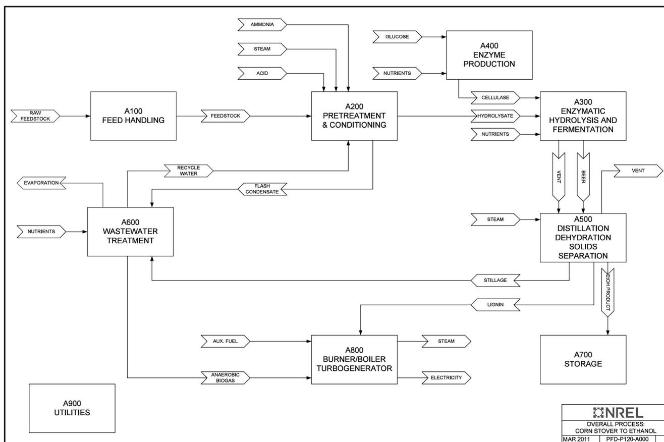
Fig. 1 Ethanol production process reprinted with permission from the National Renewable Energy Laboratory [18]
