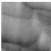
Fig. 11. Atomic force micrographs of the Vycor and Nanosil membranes (from [27]).
