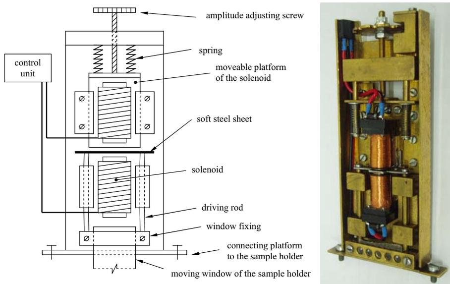
Fig. 3. The electromechanic mover
