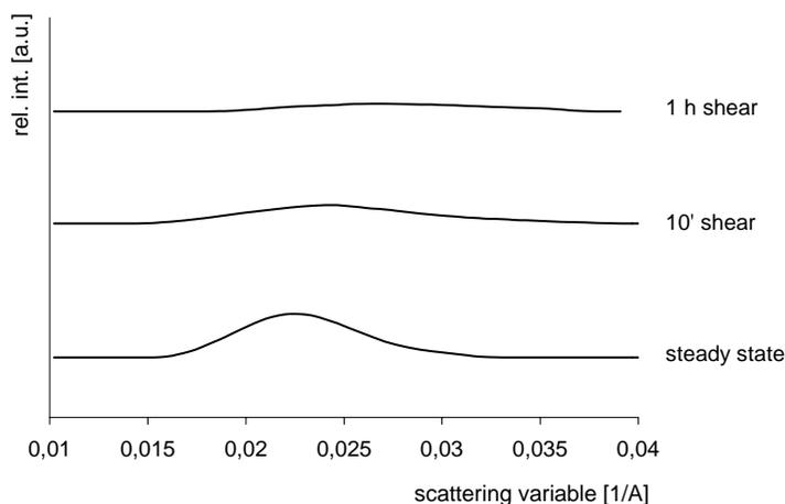
Fig. 6. 6 SAXS patterns during shear at 60 °C
