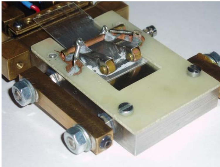
Fig. 2. The sample holder for freeze fracture
