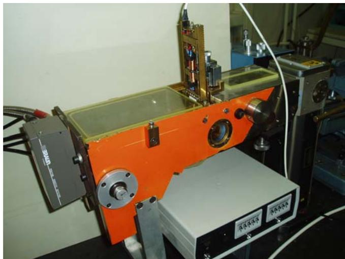
Fig. 4. The modified Kratky camera with the shear cell
