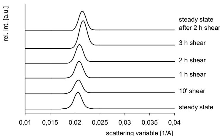
*Fig. 5.* SAXS patterns during shear at 20 °C
