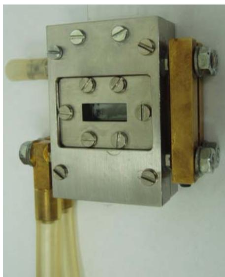
*Fig. 1.* The sample holder for SAXS
