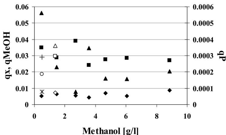
Fig. 2. Specific kinetic rates in the function of methanol. ◆  $q_x$  [1/h]; ◇  $q_{\text{MeOH}}$  [g MeOH/g CDW/h]; ▲  $q_p$  [g HSA/g CDW/h]; ■ bench top reactor; □ 19 litres stirred tank reactor; \*  $q_x$  [1/h] in 19 litres air-lift reactor; ○  $q_{\text{MeOH}}$  [g MeOH/g CDW/h] in 19 litres air-lift reactor; +  $q_p$  [g HSA/g CDW/h] in 19 litres air-lift reactor
