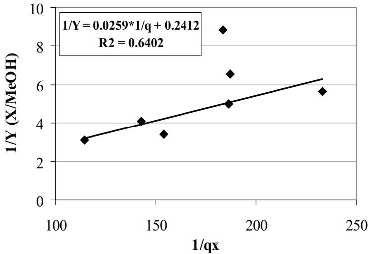
Fig. 4. Reciprocal of the cell yield in the function of reciprocal of the specific growth rate for bench top reactors
