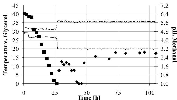
Fig. 1. Example for recombinant *P. pastoris* GS115 Mut<sup>S</sup> fermentation with direct methanol concentration control in the 65<sup>th</sup>–105<sup>th</sup> hour range. ■ Temperature [°C]; — pH; glycerol concentration [g/L]; ♦ methanol concentration [g/L]
