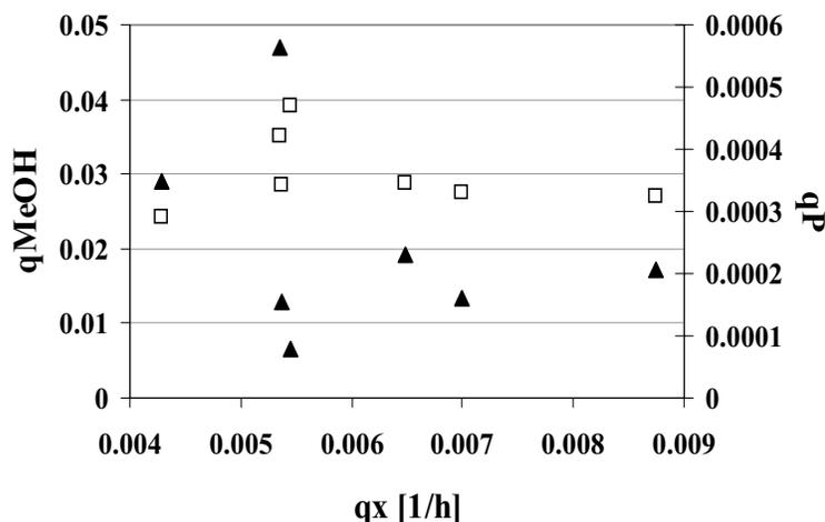
Fig. 3. Specific methanol consumption and product formation rate in the function of specific growth rate for bench top reactors.  $\blacktriangle$   $q_{MeOH}$  for bench top reactors [g MeOH/g CDW/h];  $\square$   $q_P$  for bench top reactors [g HSA/g CDW/h]
