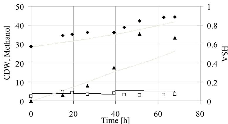
Fig. 6. Predicted and measured values of statistical model run of a fed-batch *P. pastoris* GS115 Mut<sup>S</sup> HSA fermentation. - - - predicted cell dry weight [g/L]; ◆ measured cell dry weight [g/L]; — predicted methanol concentration [g/L]; ▲ measured methanol concentration [g/L]; ··· predicted human serum albumin concentration [g/L]; □ measured human serum albumin concentration [g/L]
