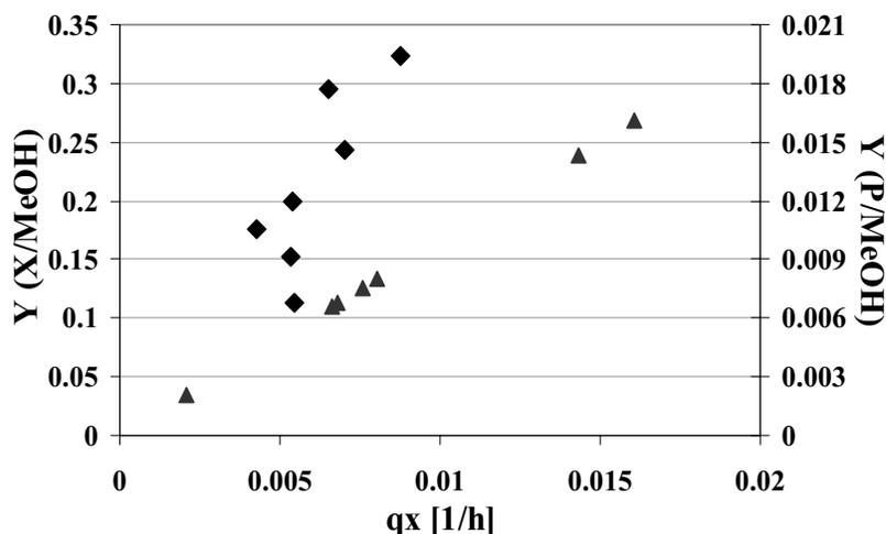
Fig. 5. Yields in the function of specific growth rate. ◆  $Y_{X/MeOH}$  for bench top reactors [g DCW/g MeOH]; ▲  $Y_{P/MeOH}$  for bench top reactors [g HSA/g MeOH]
