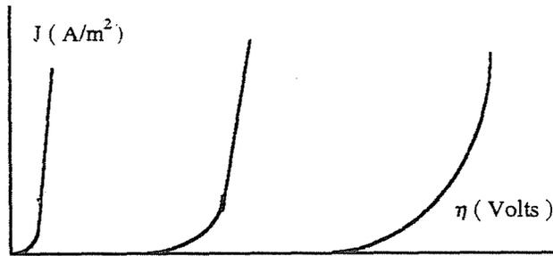
Fig. 1. Overpotential of H<sub>2</sub> evolution on various cathode metals
