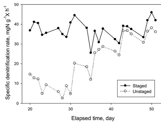
Fig. 8. Specific denitrification rates measured in the differently arranged experimental systems
