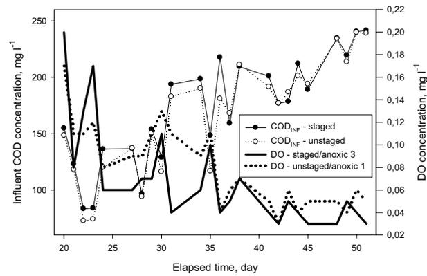
Fig. 7. Impact of the COD concentration in the mixture entering the first reactors of the systems on the DO concentrations in the unstaged anoxic reactor and in the 3<sup>rd</sup> anoxic reactor of the staged system.
