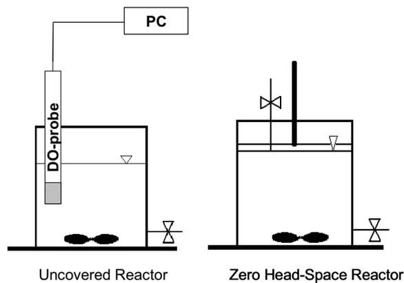
*Fig. 1.* Batch experimental setup with the uncovered and the zero-head-space reactors
