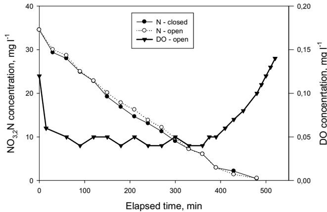
Fig. 2. Results of the batch experiment with substrate in excess ( $MLVSS_{INI, closed} = 600 \text{ mg l}^{-1} \text{ COD}$ ,  $MLVSS_{INI, open} = 660 \text{ mg l}^{-1} \text{ COD}$ ).
