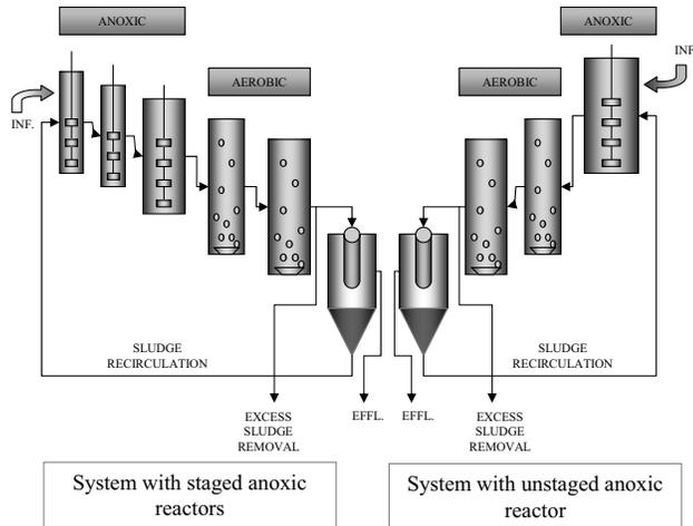
Fig. 5. Layout of the continuous-flow experiment
