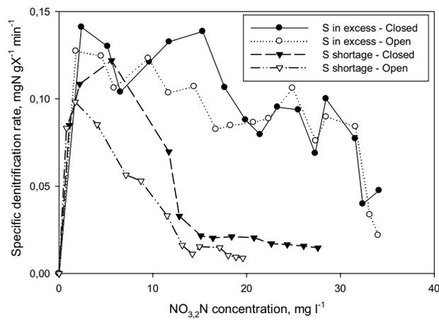
Fig. 4. Measured denitrification rates in the experiments with substrate in excess and substrate shortage
