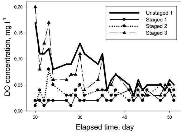
Fig. 6. Dissolved oxygen concentrations measured in the anoxic basins of the experimental systems
