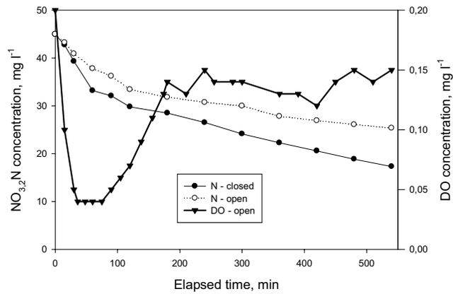
Fig. 3. Results of the batch experiment with substrate shortage ( $MLVSS_{INI, closed} = 1450 \text{ mg l}^{-1} \text{ COD}$ ,  $MLVSS_{INI, open} = 1160 \text{ mg l}^{-1} \text{ COD}$ ).
