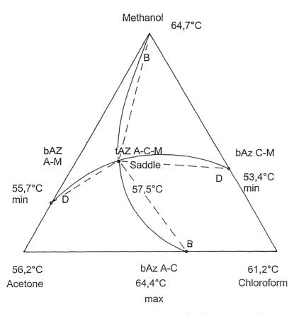
Fig. 1. Azeotropic points and their characteristics, distillation regions, boundaries and their approximation by the konovalov's rule (B - bottom product, D - distillate product, bAz - binary azeotrope, tAz - ternary azeotrope)
