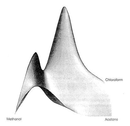
Fig. 5. 3D-view of the driving forces for the batch distillation of the mixture acetonechloroform-methanol (1 bar)
