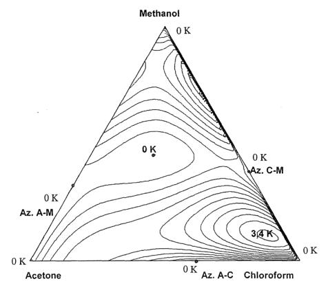
Fig. 6. Driving forces isolines for the batch distillation of the mixture acetone-chloroform-methanol (1 bar)
