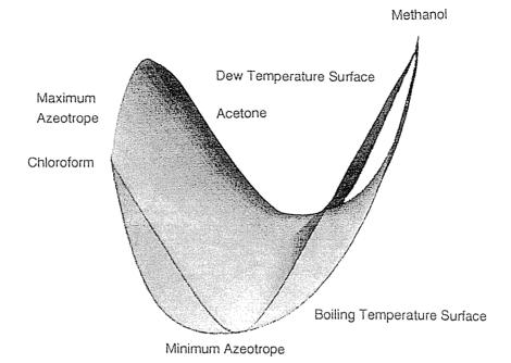
Fig. 4. Equilibrium diagram for the ternary mixture acetone- chloroform-methanol (1 bar)
