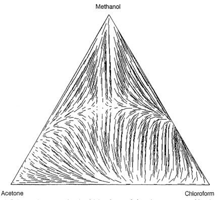
Fig. 7. Inference lines map for the driving forces of the mixture acetone-chloroformmethanol (1 bar)
