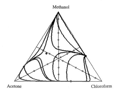
Fig. 2. Residue curve map for the mixture acetone-chloroform-methanol (1 bar, azeotrope points are designed by.)
