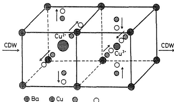
Fig. 2. The changes of the oxygen-environment around the Cu-ions having different valency
