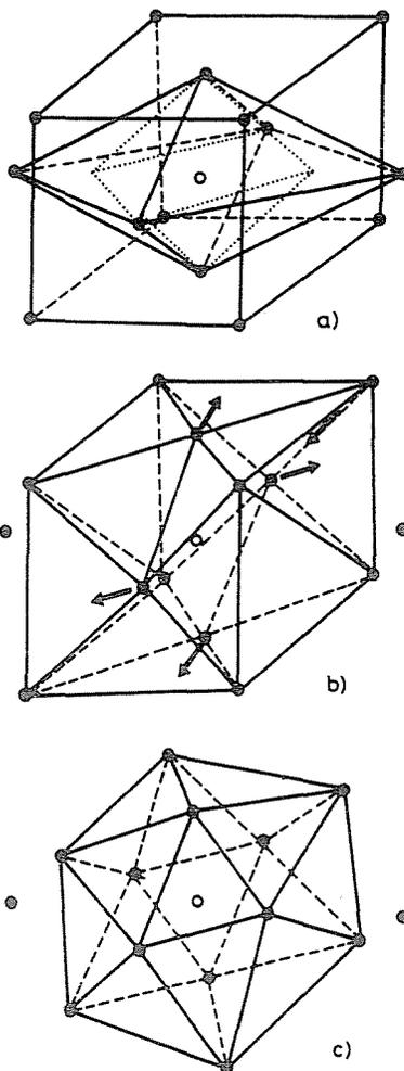
*Fig. 1.* a) An orthorhombic cell of the high  $T_c$  superconductors perovskite structure showing basic cube and elongated octahedron. At the centre of these octahedron is the copper atom (not shown); b) Same structural arrangement as (a) but highlighting the icosahedral five-fold co-ordination (chemical bonding) for atoms in the basic cell; c) The icosahedral co-ordination 'cell' formed by displacements indicated in (b)
