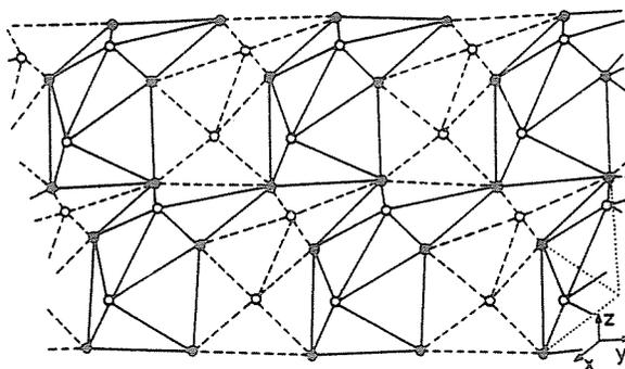
Fig. 3. A schematic of the proposed 3-dimensional icosahedral (solid lines) to non-icosahedral (dotted) breathing displacements of oxygen atoms in perovskite-type materials (o-oxygen; o-Ba(La)Y). Note the two-dimensional planar warping, proposed previously by Mattheiss and others (Proc. Int. Conf. on High  $T_c$  (1988); Mattheiss (1987); Jorgensen (1987); Inderhees (1988); Tuominen (1988); Chang-feng (1987); Inoue (1987)), can be observed
