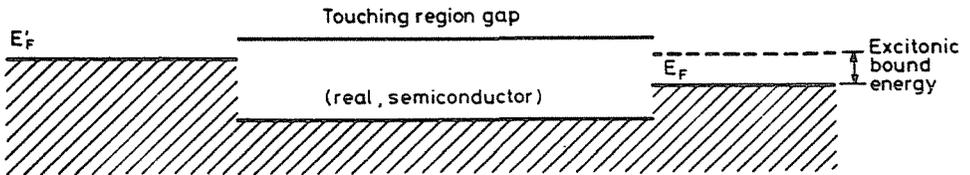
Fig. 4. The schematic diagram of the touching-region caused by the Fermi-surface—Jones-zone interaction. In the touching positions a real semiconductor gap are created, while in their neighbourhood the Fermi-surface is free in localised disjunct areas
