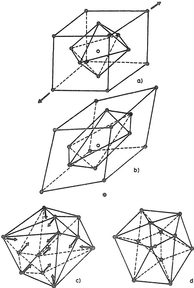
Fig. 6. The changes of the Frank-Kasper coordination polyhedra in a mechanically distorted perovskite structure: a) Non-distorted perovskite; b) Diagonally elongated perovskite by external mechanical stresses; c) The Frank-Kasper coordination polyhedra in the distorted case very close to a distorted icosahedron
