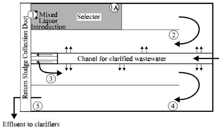
*Fig. 1.* Schematic of the flow-through activated sludge basin demonstrating the installation of a selector in Train I
