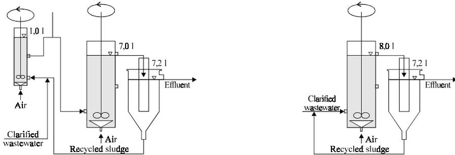
Fig. 2. Arrangement of the system with the aerobic selector and the reference system containing no selector
