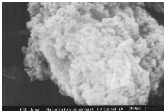
Fig. 2. SEM image of SiO 2 sample (obtained at ph = 1 and 80 °C)
