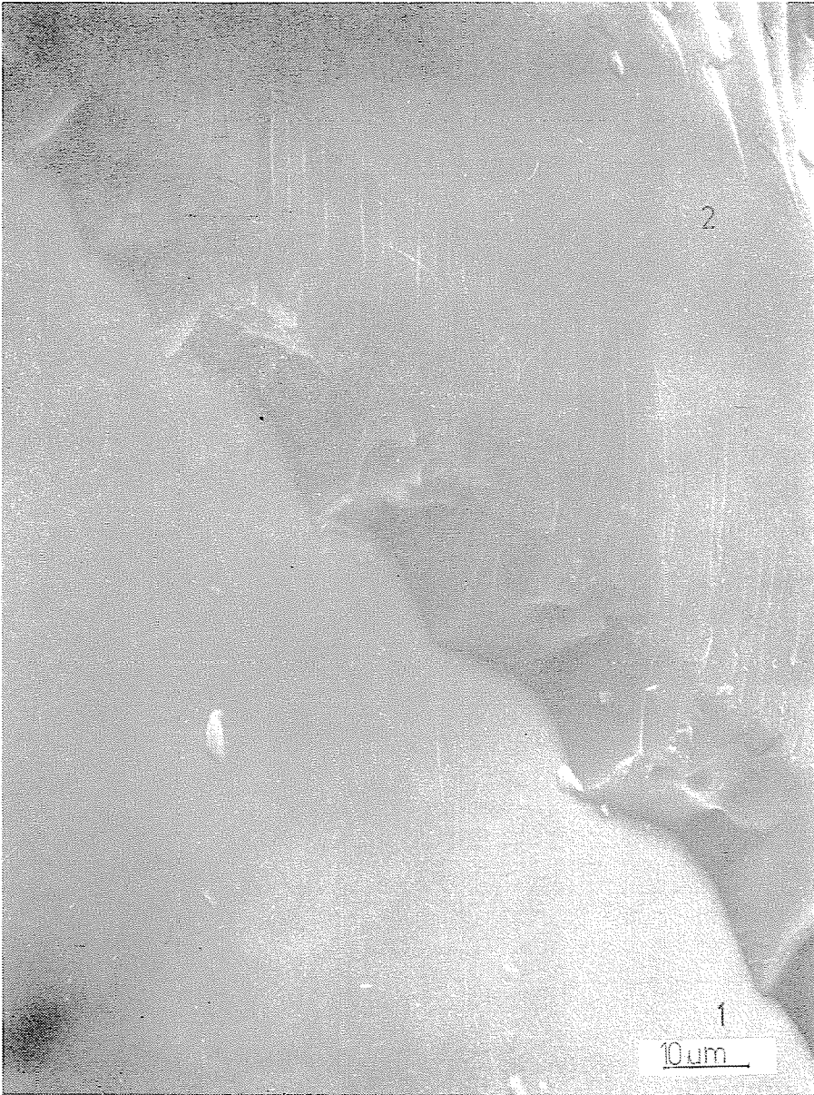
Fig. 21. Scanning electronmicrograph of the phase boundary between electrocorundum (1) and ceramic bonding material melt (2)
