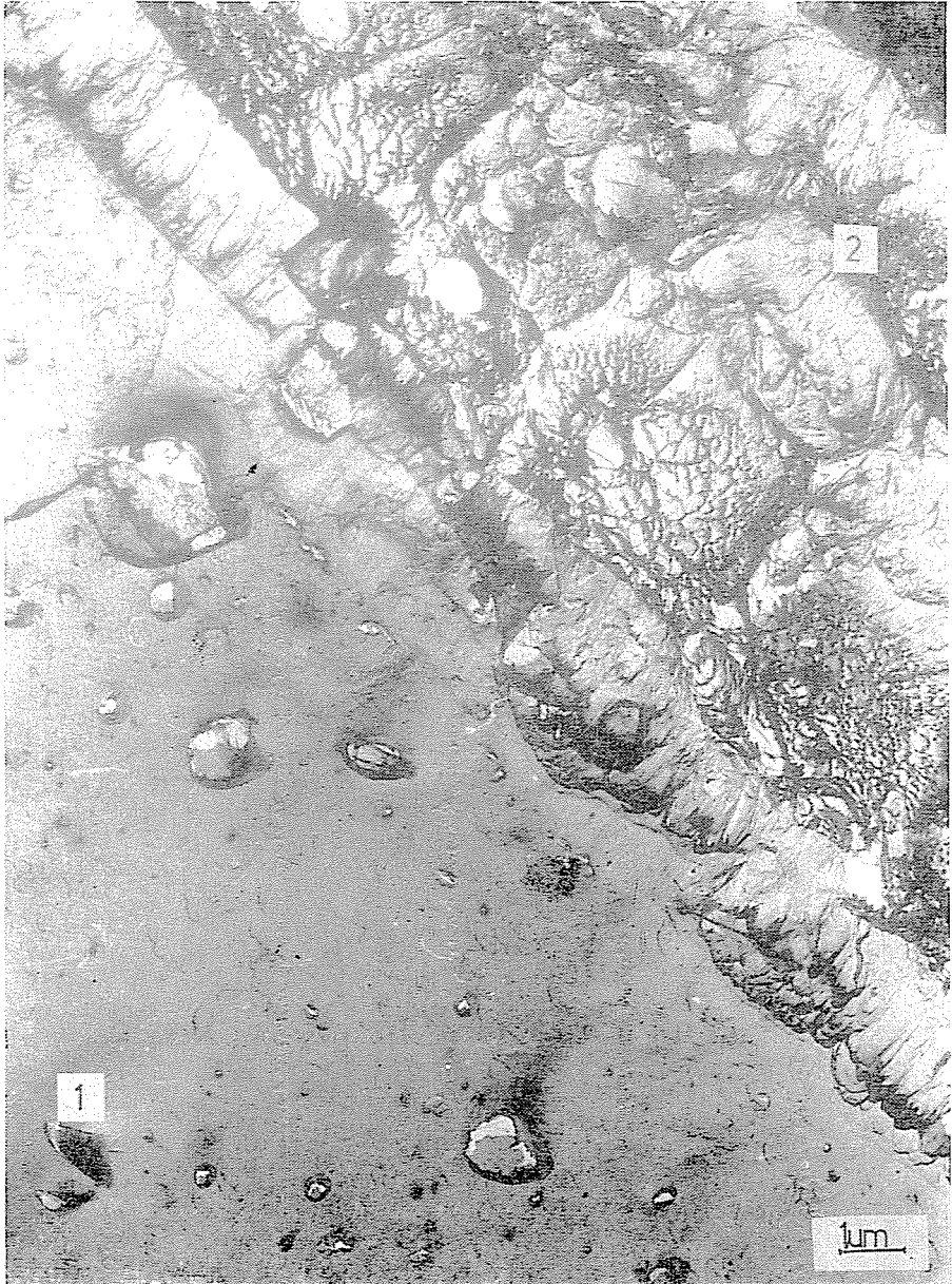
Fig. 22. Electron microscope image of the phase boundary between electrocorundum (1) and ceramic bonding material melt (2)
