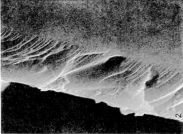
Fig. 18. Scanning electron micrograph of a silicon carbide grinding grain (1) and ceramic bonding material (2). \times 5000
