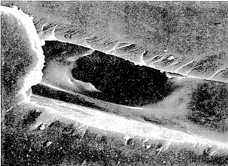
Fig. 17. Scanning electron micrograph of the phase boundary of a silicon carbide grinding grain (1) and ceramic bonding material (2). \times 1600
