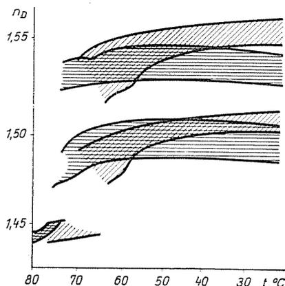
Fig. 7. Refractive indices vs. temperature curves of two principal groups of fractions obtained by the separation on silica gel of Sample 3. Oblique shaded lines show extension of the set of curves relating to fractions between the first and tenth, horizontal shaded lines show that of the set of curves relating to fractions between the eleventh and fifteenth fraction
