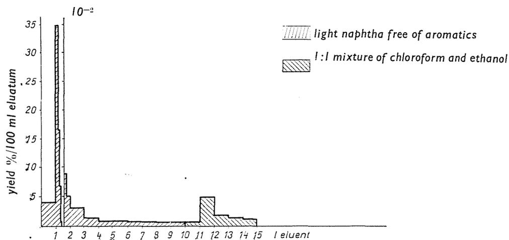
Fig. 1. Chromatogram of the separation, on silica gel, of Sample 1
