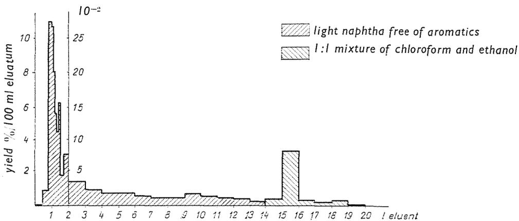
Fig. 3. Chromatogram of the separation, on silica gel, of Sample 3
