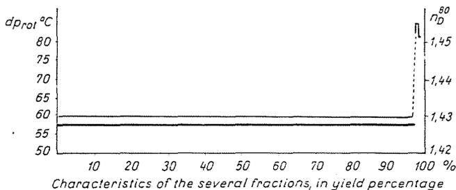
Fig. 5. Setting points and refractive indices of hydrocarbons separated by chromatography, from Sample 2\*; — rotational setting point, - - -  $n_D^{80}$ , measured
