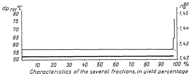
Fig. 4. Setting points and refractive indices of hydrocarbons separated by chromatography, from Sample 1; — rotational setting point, - - -  $n_D^{80}$ , measured
