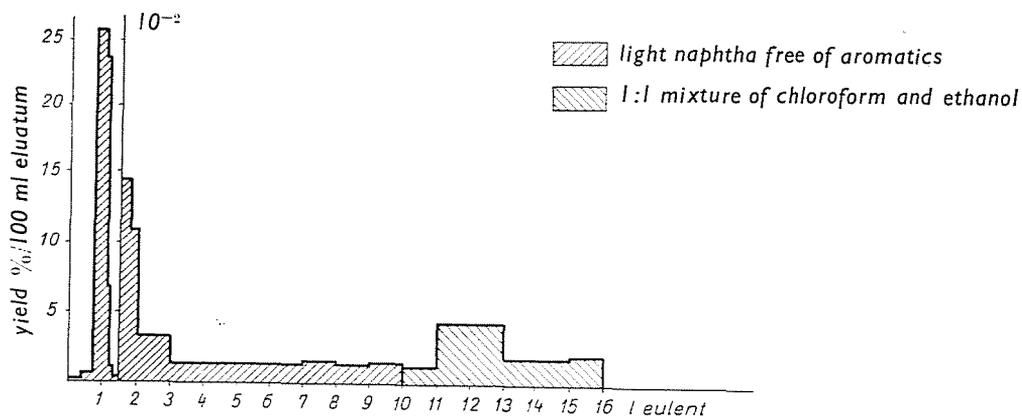
Fig. 2. Chromatogram of the separation, on silica gel, of Sample 2
