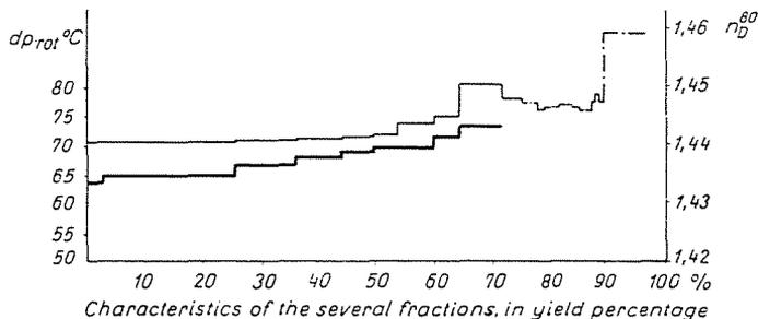
Fig. 6. Setting points and refractive indices of hydrocarbons separated by chromatography, from Sample 3\*\*; — rotational setting point, - - -  $n_D^{80}$  measured, ·····  $n_D^{80}$  calculated
