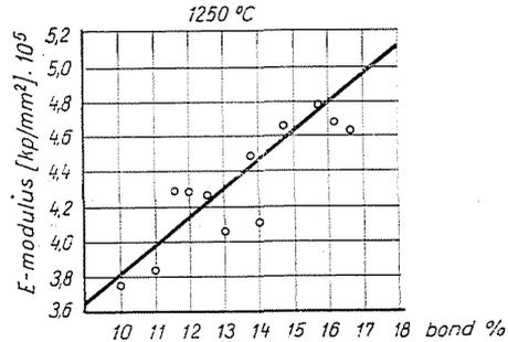
Fig. 13. Moduli of elasticity of grinding tools ignited at 1250 °C, as a function of binder quantity
