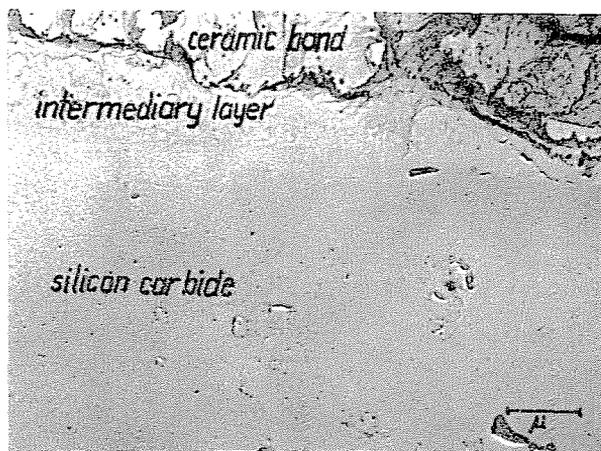
Fig. 10a. The binding characteristics of the ceramic binding material and silicon carbide grains.  $\times 15000$
