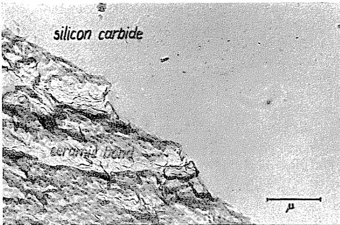
Fig. 10c. The binding characteristics of the ceramic binding material and silicon carbide grains;  $\times 21000$
