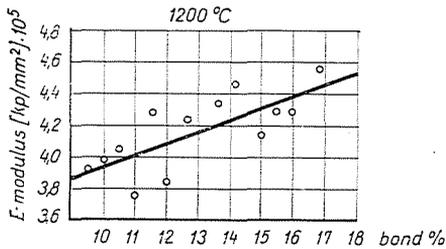
Fig. 12. Moduli of elasticity of grinding tools ignited at 1200 °C, as a function of binder quantity
