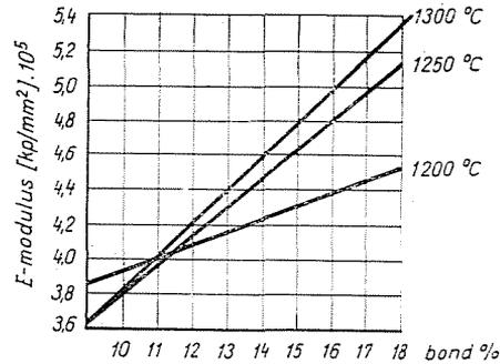
Fig. 15. Effect of ignition temperature upon the modulus of elasticity
