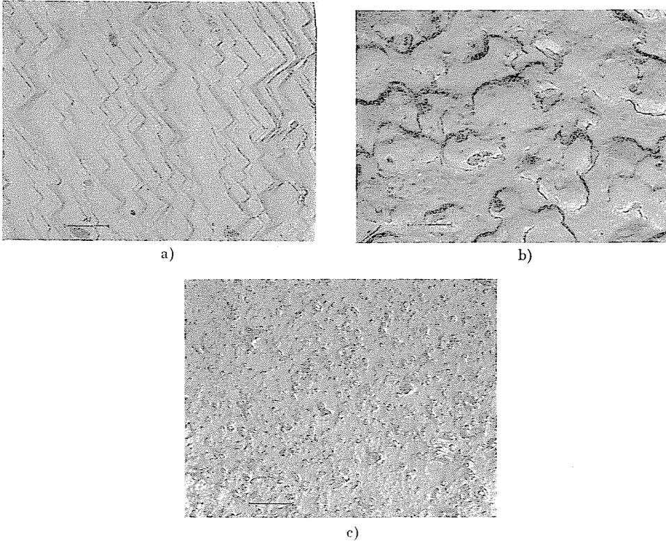
Fig. 7. Electron microscopy of normal corundum grains;  $\times 16\ 500$
