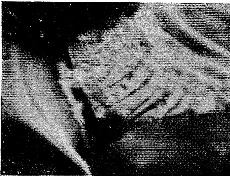
*Fig. 9.* Longitudinal creases in binder bridges, magn.  $\times 900$
