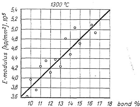
Fig. 14. Moduli of elasticity of grinding tools ignited at 1300 °C, as a function of binder quantity
