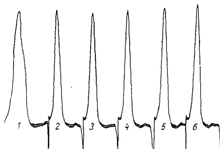
Fig. 1. The Br K\alpha lines of gasolines with a content of 2.5 ml TEL/litre, originating from the six fields
