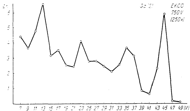
Fig. 23. Gamma spectrum of activated gallium contaminated by Zn [Ga(2)] on 750 V
