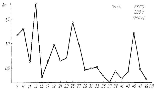
Fig. 15. Gamma spectrum of activated "pure" gallium [Ga(4)] on 800 V
