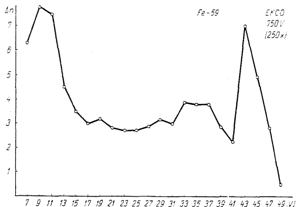
Fig. 21. Gamma spectrum of ^{59}\text{Fe} on 750 V
