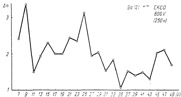
Fig. 13. Gamma spectrum of activated gallium contaminated by zinc [Ga(2)] on 800 V
