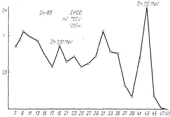
Fig. 8. Gamma spectrum of 65 Zn on 750 V
