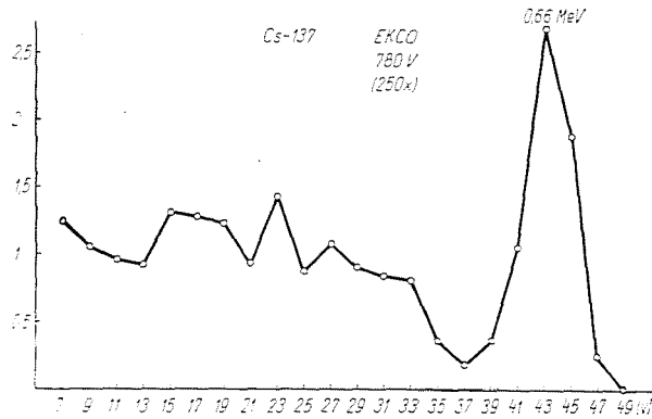
Fig. 4. Spectrum of ^{137}\text{Cs} on 780 V
