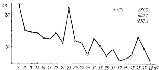
Fig. 14. Gamma spectrum of activated gallium contaminated by zinc [Ga(3)] on 800 V
