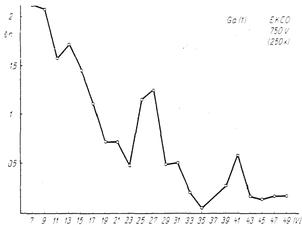
Fig. 22. Gamma spectrum of active "pure" gallium [Ga(1)] on 750 V
