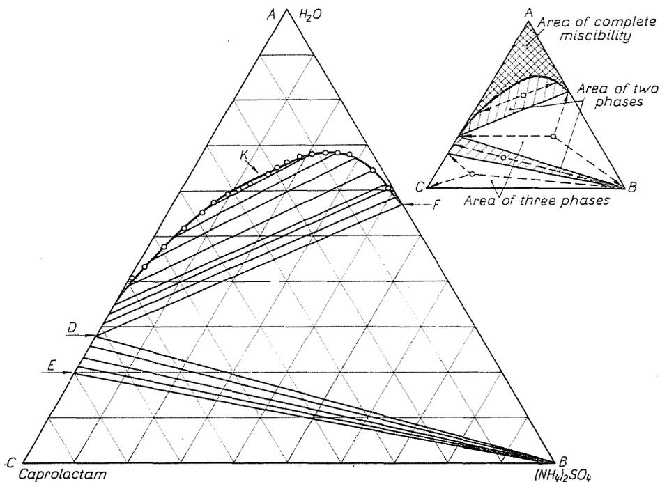
Fig. 1. The system ammonium sulphate/caprolactam/water at 20° C
