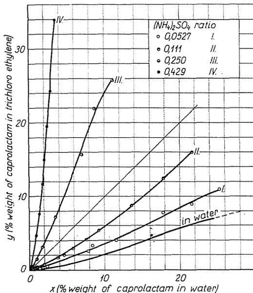
Fig. 5. Equilibrium diagram ( $x$  vs  $y$ ) of the system caprolactam/water/ammonium sulphate/trichloro ethylene
