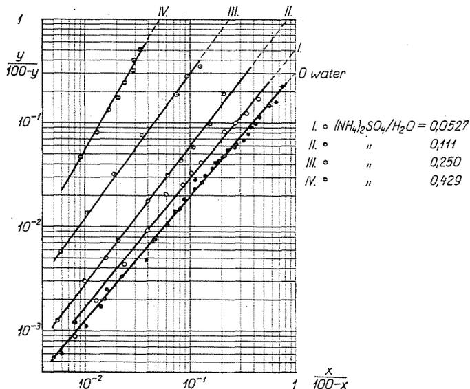
Fig. 4. Diagram after Hand, of the system water/ammonium sulphate/caprolactam/ trichloro ethylene
