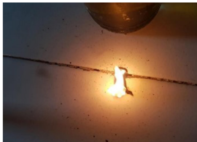
Fig. 7 Burn test on black phase bio-oil product
