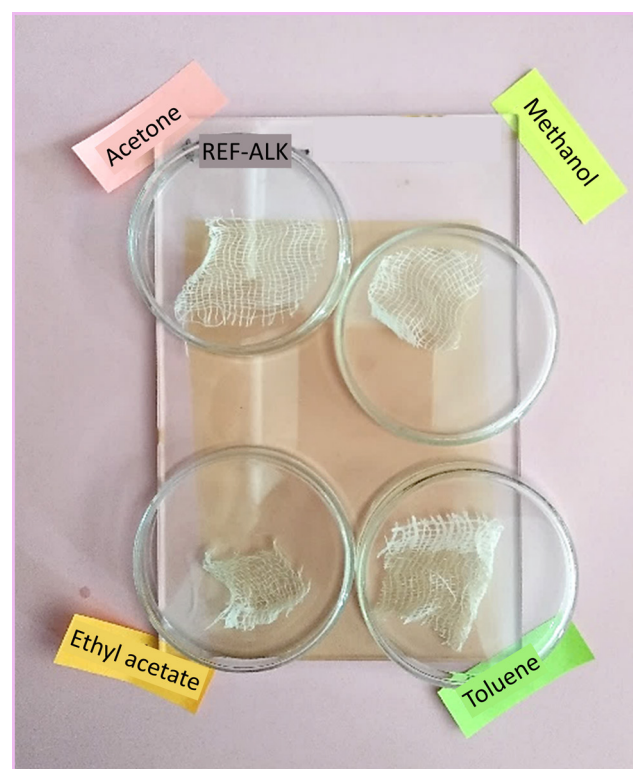
Fig. 11 The application of the solvent resistance test
