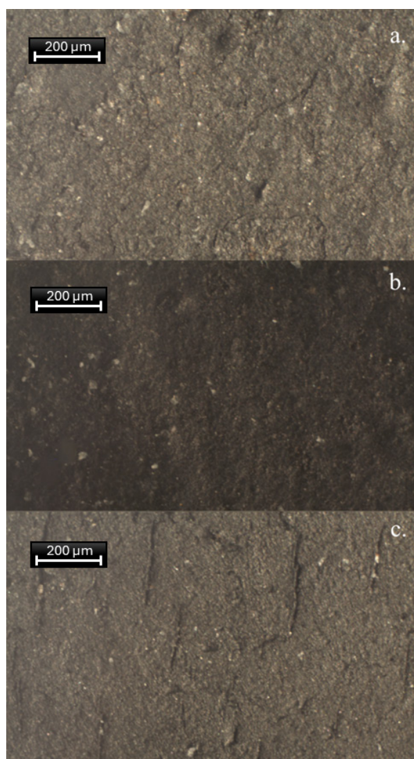
Fig. 1 Microscopic observation of tyre samples after (a) 0 min, (b) 360 min, and (c) 1080 min of UV irradiation
